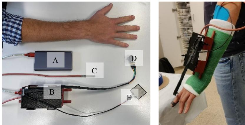
**Fig. 4.** Protocast 1.0 test setup. A. Power bank, B. Processing unit, C. PT100 temperature sensor, D. Heart rate monitoring sensor, E. FSR pressure sensor, Muscle activity sensor is not shown in the image.
