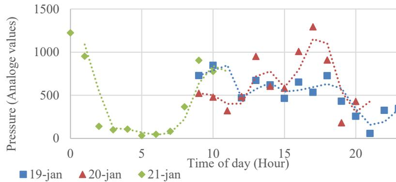
**Fig. 11.** Average hourly cast pressure during the day. The moving average is indicated by the dotted line. Data compared per day.
