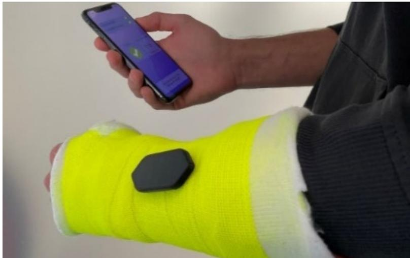
**Fig. 1.** Patient reading healing data from his smartphone. Data is collected by the SMC and transmitted wirelessly for analysis.
