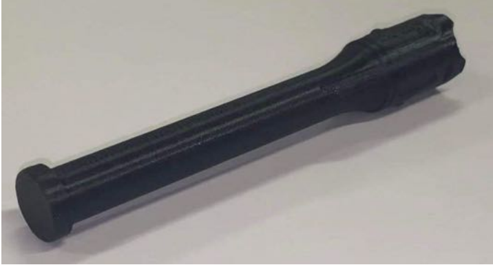
Figure 1: FDM printed model of NASA’s sample tube to test gripper compatibility
