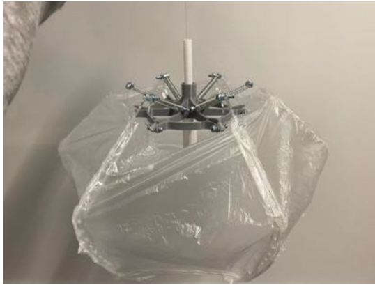
Figure 6: The final state of the prototype with the plastic bag simulated the net functionality.
